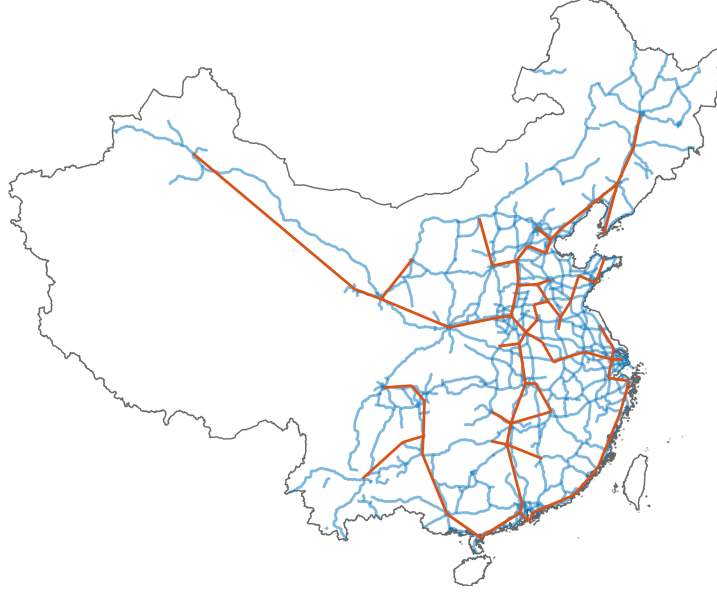
Figure 4: The Minimum Spanning Tree for the 2010 Expressway Network Note: The minimum spanning tree is constructed as the network with the minimum total length that connects the 55 major cities that are on the actual 2010 expressway network.
