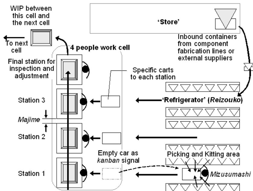
Figure 7. The pulling of materials flow in the cell production system
