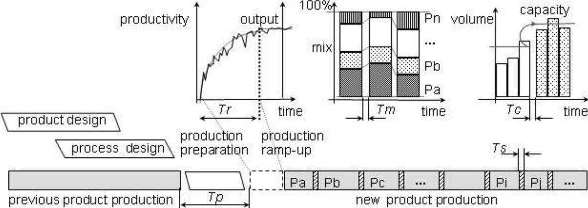
Figure 1. Production system under dynamic conditions.
