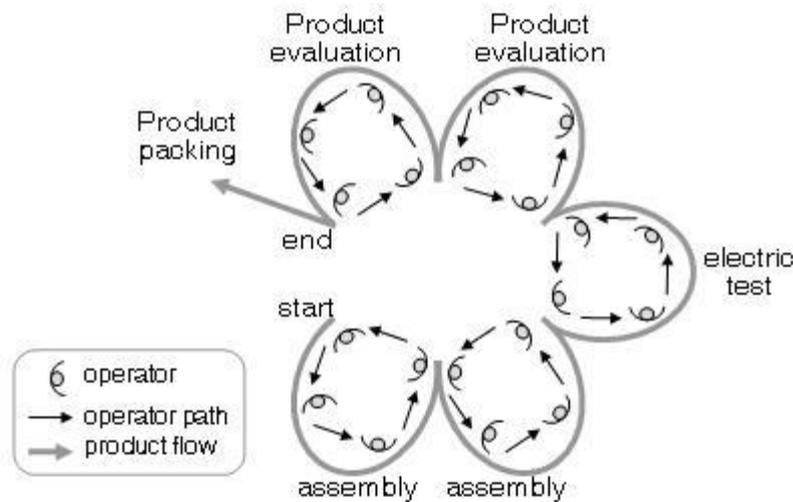
Figure 6. Work cells arranged in the format of a flower.
