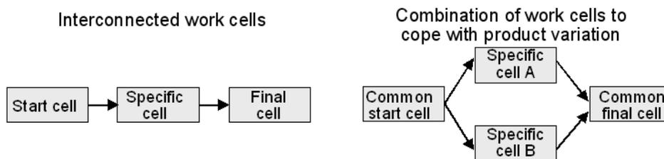
Figure 5. Different patterns of work cells interconnection
