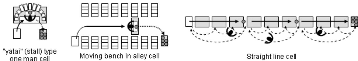
Figure 3. Different patterns of work cells
