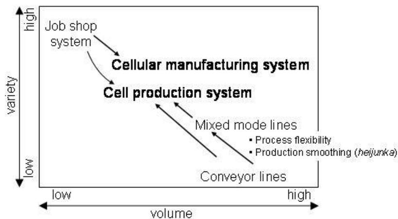
Figure 2. Trajectories towards cellular manufacturing and cell production system
